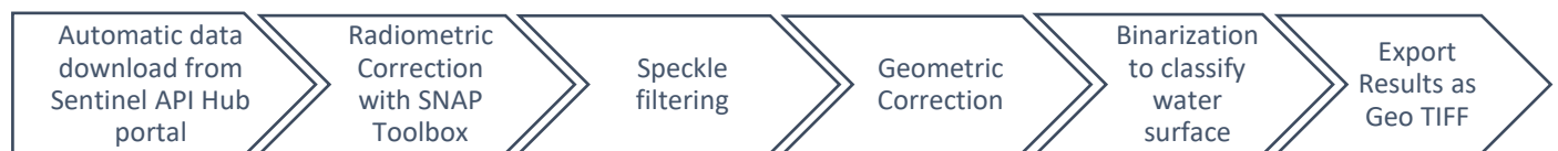
Figure 3: Procedure for acquisition of waterbodies
