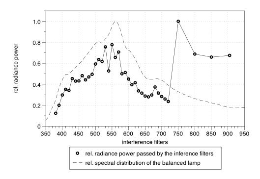
Figure 3.12: The balanced lamp used for the spectral response measurement.
