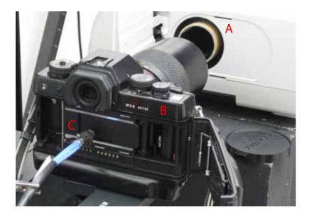
**Figure 3.6:** The used setup to evaluate the angle dependency of the interference filters. With  $\bf A$  camSPECS,  $\bf B$  35 mm camera with open back,  $\bf C$  spectrometer fiber-optics.
