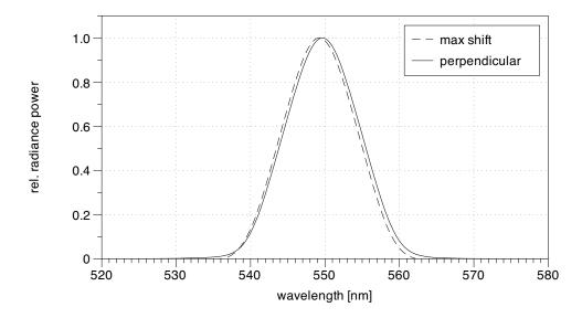
**Figure 3.5:** Two spectral power distribution measurements of the 550 nm filter. One placed in the corner of the image (dashed line) the other with the filter placed in the center of the image (solid line).
