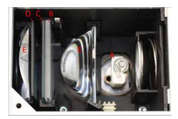
Figure 3.7: The optical system of the projector.
