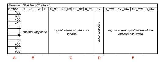
Figure 5.2: The results txt-file of the spectral response modul.
