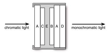
Figure 2.3: A complete interference filter.
