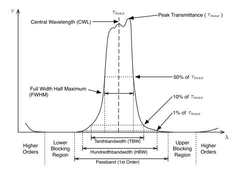
Figure 2.4: Interference filter parameters.
