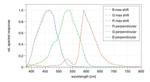
**Figure 3.4:** The spectral response of the Nikon D70 (scaled to unity) measured with the maximum possible shift (dashed lines) and with the camera mounted perpendicular to the inference filter (solid lines).
