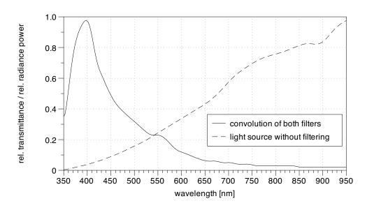
Figure 3.11: Convolution of both filters (solid line) and the light source without filters (dashed line).
