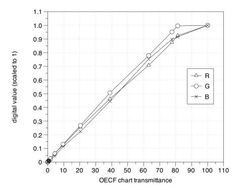
Figure 4.2: An sample OECF showing highlight-compression
