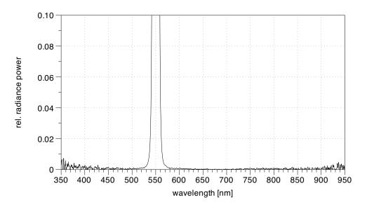
Figure 3.3: Noise of the HR4000 spectrometer.
