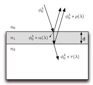
Figure 2.1: Interference at a thin layer.
