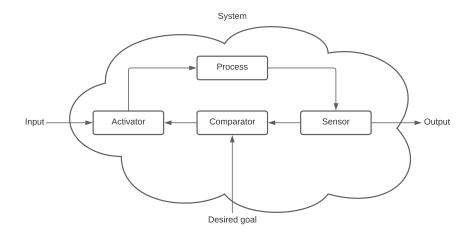
Figure 4.4: A Closed-Loop Feedback System by Jackson (2019)
