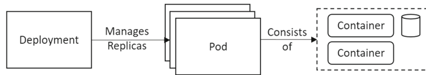
Fig. 3 A deployment defines the life cycle of a pod, which consists of one or more containers and an optional volume for information storage. Submitting a deployment to the controller instructs Kubernetes to instantiate the pod on a node and ensure its continuous availability in the cluster
