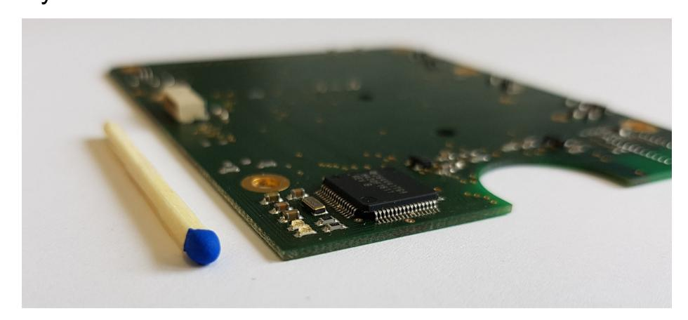
By applying very small drops of silver conductive adhesive and soldering paste, contacts can be formed between a diverse range of electronic components. Conductor tracks can also be applied to components with various different geometries. Miniaturisation will require even smaller structures in the future.
