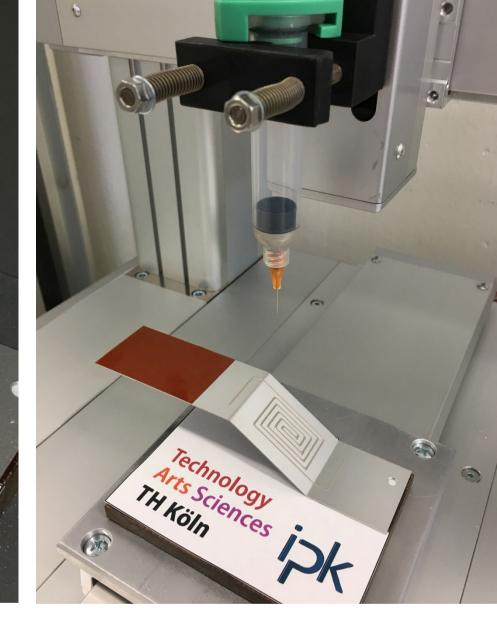
The dosing of electrically conductive adhesives is currently very limited due to the fact that they frequently contain silver particles. These particles, which can have a diameter of 20  $\mu$ m to 50  $\mu$ m, quickly damage or block the dosing valve due to their abrasive effect.
