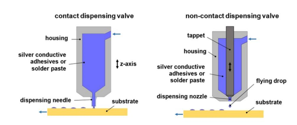
Irrespective of the dosing system, the dispensing volume is dependent on various different parameters and stable conditions can only be guaranteed within narrow limits.
